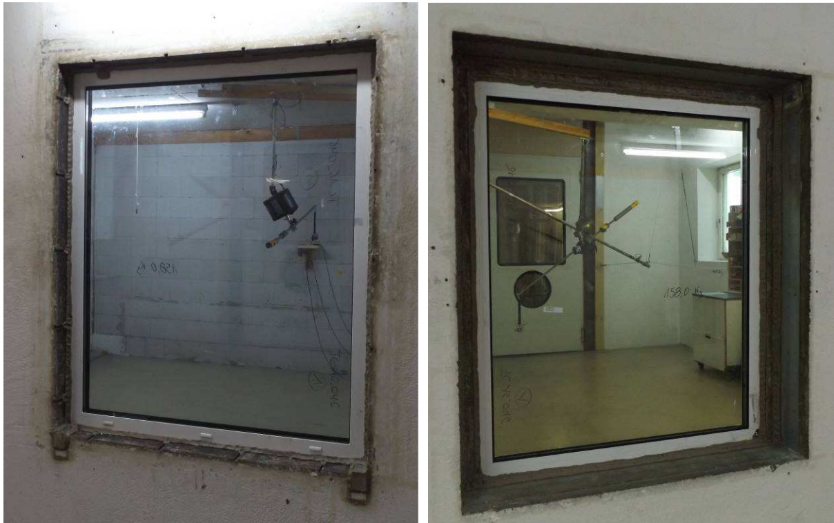
fig 1 Photo(s) of the mounted element, taken by ift Laboratory for Building Acoustics
